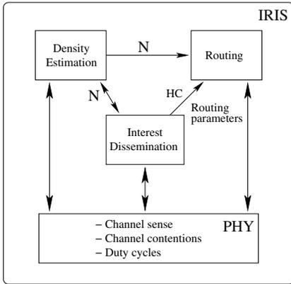
Fig. 3. A diagram of the IRIS system and its main components.
