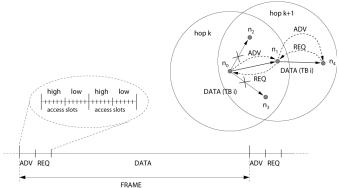
Fig. 2. ADV/REQ/DATA contention example and time frame structure.
