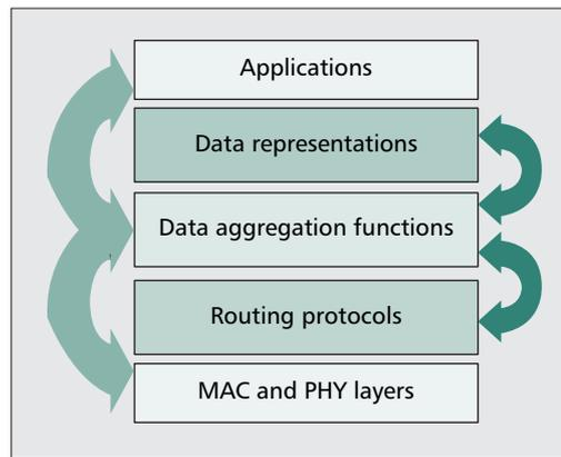
■ **Figure 1.** Diagram for in-network aggregation techniques and their relation with different protocol layers. We stress that in general data processing also interacts with the application, MAC, and PHY layers.
