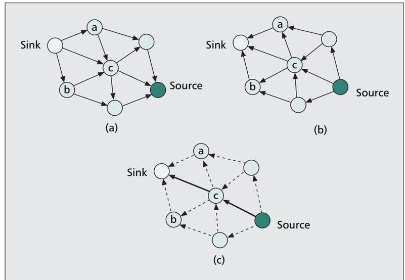
■ **Figure 2.** A simplified scheme for Directed Diffusion [1]: a) interest dissemination; b) gradients setup; c) data delivery along the reinforced path.
