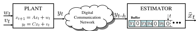
Fig. 1. Networked systems modeling. Sampled observations at the plant site are transmitted to the estimator site via a digital communication network. Due to retransmission and packet loss, observation packets arrive at the estimator site with possibly random delay.
