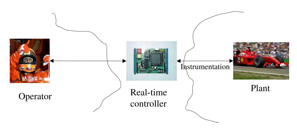
A real-time controller is a computer based system, which produces results to inputs complying with some temporal constraints
