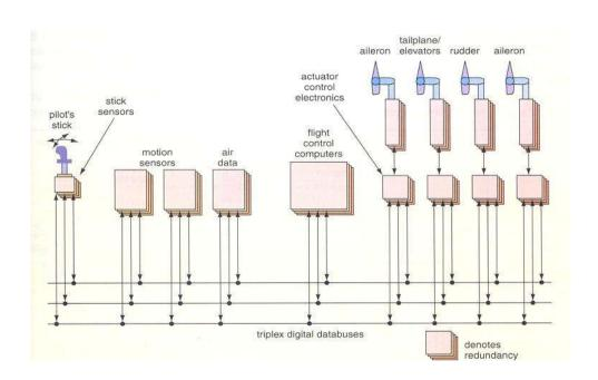
Distributed: computation is distributed across different nodes which communicate by means of a bus
