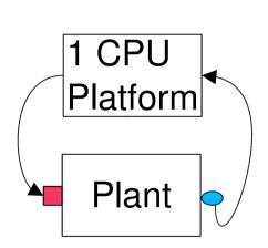
Single node: computation is concentrated in one node, which has direct access to sensors and actuators
