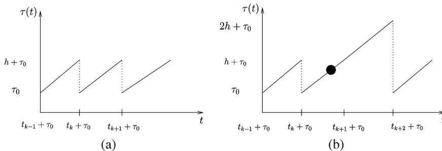
**Fig. 10.** Variable delay in NCS for constant network delay  $\tau_k = \tau_0$ ,  $\forall k \in \mathbb{N}$  and periodic sampling with period  $t_{k+1} - t_k = h$ ,  $\forall k \in \mathbb{N}$  for: (a) no packet dropout and (b) one packet dropout.
