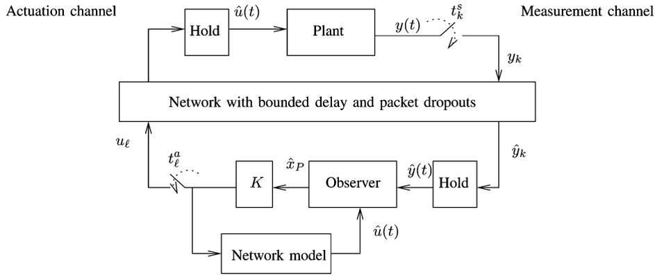
**Fig. 11. Two-channel feedback NCS with observer-based controller.**
