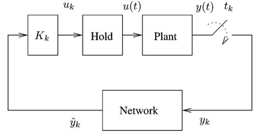
Fig. 13. One-channel feedback NCS with switching controller.
