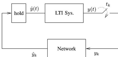
Fig. 4. One-channel feedback NCS with LTI plant/controller.
