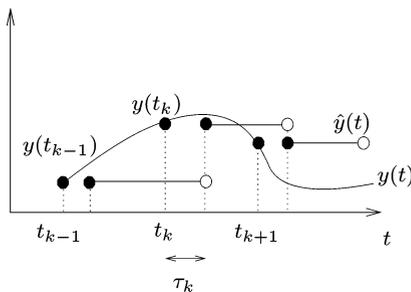
**Fig. 6.** Piecewise constant signal  $\hat{y}(t)$  defined by (14).
