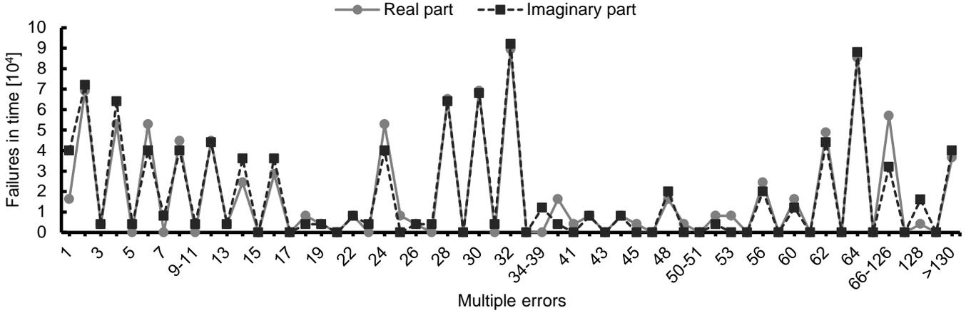
Fig. 3. FFT real and imaginary parts multiple output errors FIT. Consecutive distributions that were never experimentally observed are grouped in the picture (for instance, 9 to 11 errors, and 20 to 21). Statistical error is limited to 5%.
