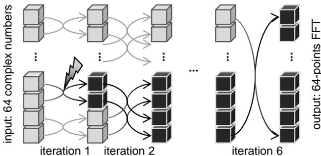
Fig. 2. Graphical representation of the FFT algorithm under radiation. At each iteration, a thread updates two-by-two all the 64 values of the FFT using the basic butterfly module. Six iterations are necessary to complete the execution. If an operation in one iteration is corrupted by radiation, two (or more) values will be wrongly updated, and the number of errors will double in the following iteration.
