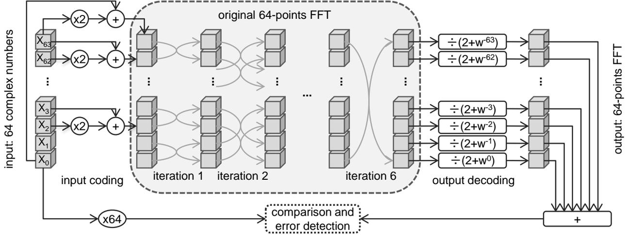
Fig. 4. FFT hardening scheme. The 64 complex elements of the input are coded, then the 64-point FFT is performed with the original algorithm, and its output is decoded. Errors are detected comparing the checksum generated summing the output values with  $X_0 \times N$ .
