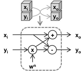
Fig. 1. A basic butterfly module used to update two-by-two all the 64 elements composing the FFT.
