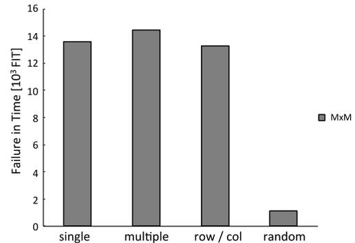
Figure 5:  $MxM$  output errors patterns FIT at NYC when executed with double data.
