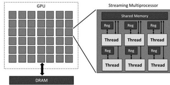
Figure 1: Simplified internal structures of a GPU.
