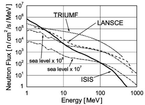
**Figure 4: ISIS and LANSCE spectrum compared to those of the TRIUMF facilities and to the terrestrial one at sea level multiplied by  $10^7$  and  $10^8$  [14].**
