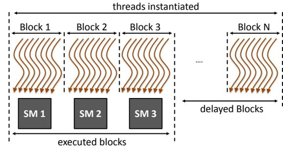
Figure 2: The instantiated threads are grouped into a grid of blocks. Each of the available Streaming Multiprocessor (SM1, SM2, and SM3) treats just one block at a time.
