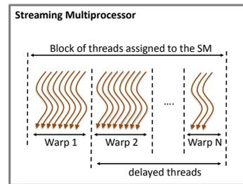
Figure 3: The block of threads assigned to a SM is divided into warps. Just one warp of threads is executed at a time in the SM.
