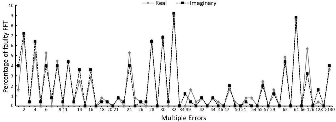
Figure 7: *FFT* real and imaginary multiple output errors percentages. Some distributions that were never experimentally observed are grouped in the picture (it is the case of 9 to 11 errors, 20 and 21 etc.). In most of the cases, the output is affected by less than 16 errors, about 32 or 64 errors. It is very unlikely to have an odd number of errors or more than 128 errors.
