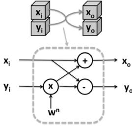
Fig. 1: A basic butterfly module used to update two-by-two all the 64 elements composing the FFT
