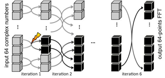
Fig. 2: In each iteration a thread updates two-by-two all the 64 values of the FFT using the basic butterfly module. 6 iterations are necessary to complete execution. If an operation in one iteration is corrupted by radiation, two (or more) values will be wrongly updated, and the number of errors will double in the following iteration.
