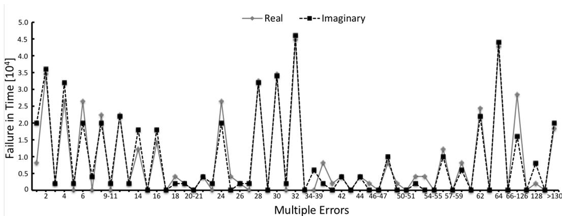
Fig. 3: FFT real and imaginary multiple output errors FIT. Consequent distributions that were never experimentally observed are grouped in the picture (it is the case of 9 to 11 errors, 20 and 21 etc.).
