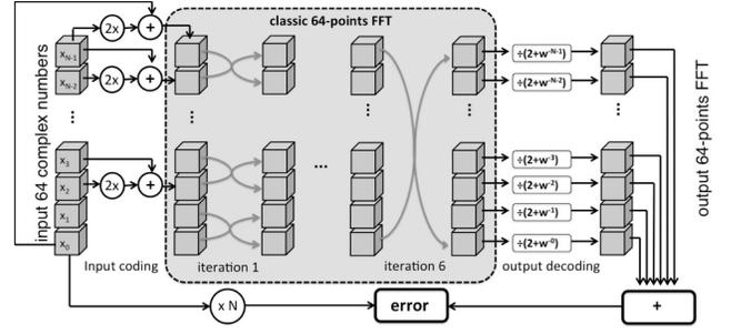
Fig. 4: FFT Hardening scheme. The 64 input complex elements are coded, then the 64-points FFT is performed with the classical algorithm, and output is decoded. Errors are detected comparing the checksum generated summing the output values with  $Nx_0$ .
