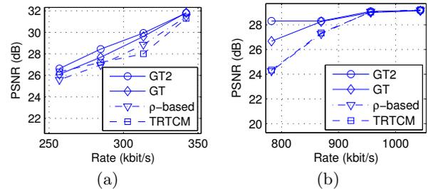
**Figure 3: Average PSNR vs. the transmission rate  $R_b$  for different sequences coded in the setting b) ( $QP = 30$ ). a) foreman b) flower.**
