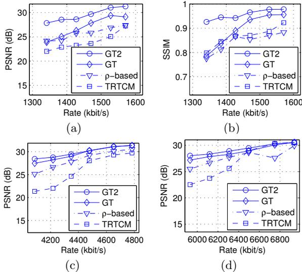
**Figure 2: Average quality metrics vs. the transmission rate  $R_a$  for different algorithms in setting a) ( $QP = 30$ ). The plots report the PSNR values for the sequences foreman (a), flower (c), mobile (d), and the SSIM value for foreman (b).**
