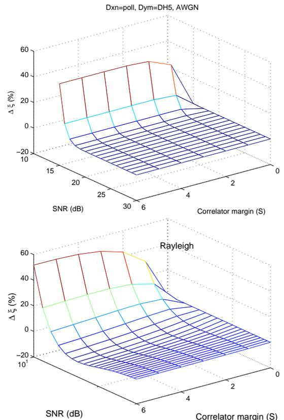
Fig. 4. Energy efficiency variation due to  $S$  (AWGN (top), Rayleigh channel (bottom),  $Dxn = POLL$ ,  $Dym = DH5$ ).
