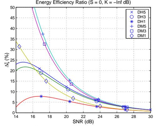
Fig. 3. Energy efficiency variation due to master-slave swapping.
