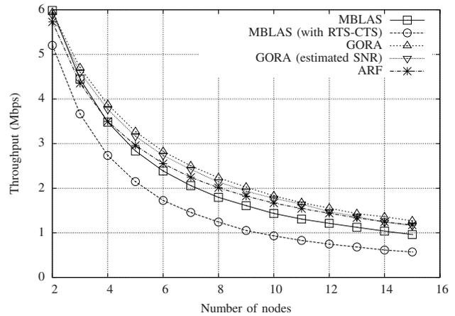
Figure 5. Throughput of rate adaptation algorithms, as a function of the total number of nodes; the test node has SNR = 10 dB.
