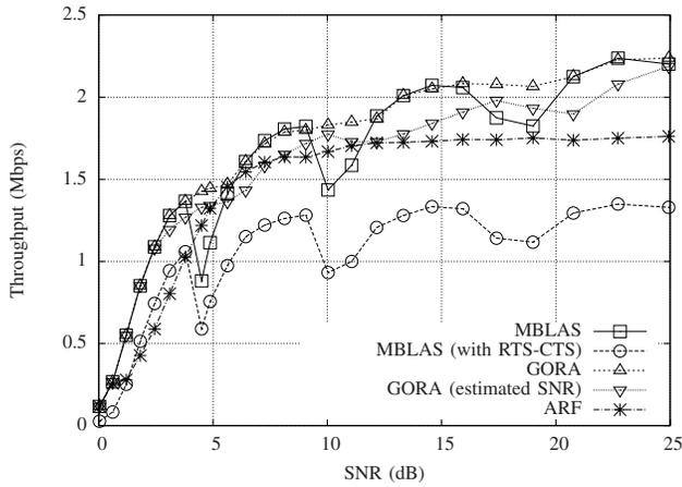
Figure 4. Throughput of rate adaptation algorithms, as a function of the SNR, in presence of 9 interfering nodes.
