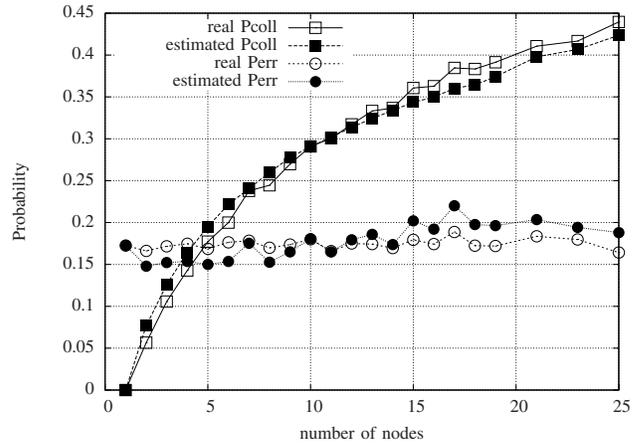
Figure 2. Actual and estimated  $P_{coll}$  and  $P_{err}$  as a function of the total number of nodes; the test node has SNR = 20.54 dB
