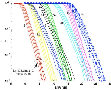
Figure 1.  $P_{err}$  vs SNR for different 802.11g PHY modes and MPDU sizes
