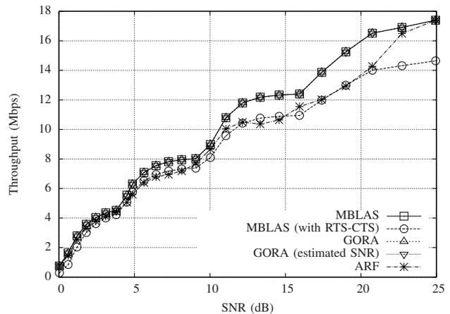
Figure 3. Throughput of rate adaptation algorithms, as a function of the SNR, in case of no interference.
