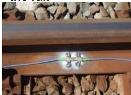
FBG soldered on the rail
