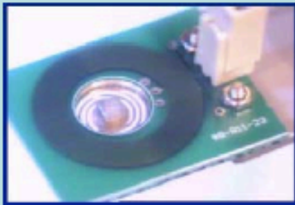
Wen J. Li et al., 2000 Chinese univ. of Hong Kong 680 \mu\text{W} , 9.5\text{g} @ 110 \text{ Hz} , 1 \text{ cm}^3
