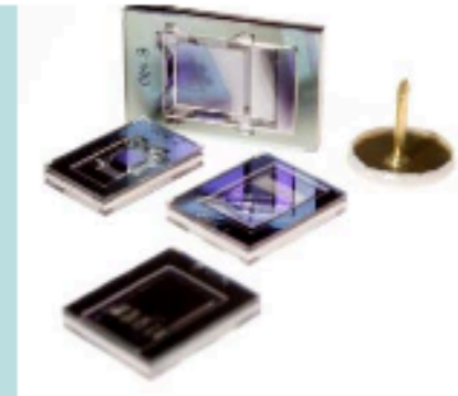
Elfrink et al., 2008n IMEC, 60 \mu\text{W} , 2\text{g} @ 572\text{Hz} , 0.2 \text{ cm}^2
