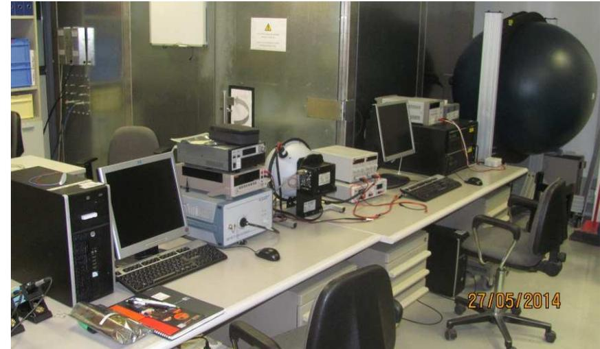
Integrating spheres for optical simulation
