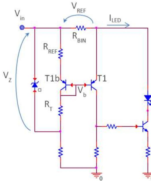
$$V_{REF} = V_{in} - V_b + V_{be}$$
