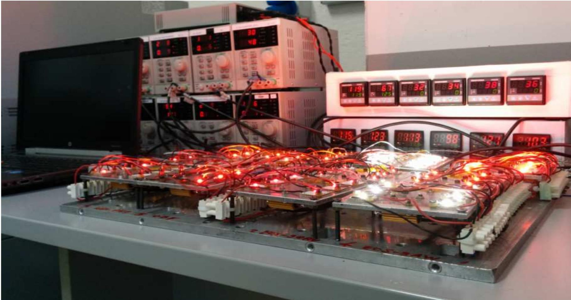
Several optical and thermal tests, life cycle simulations, quality..
