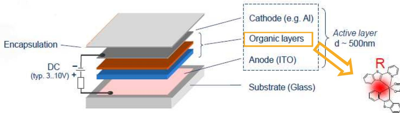
Small molecule OLED deposited through evaporation in vacuum chambers
