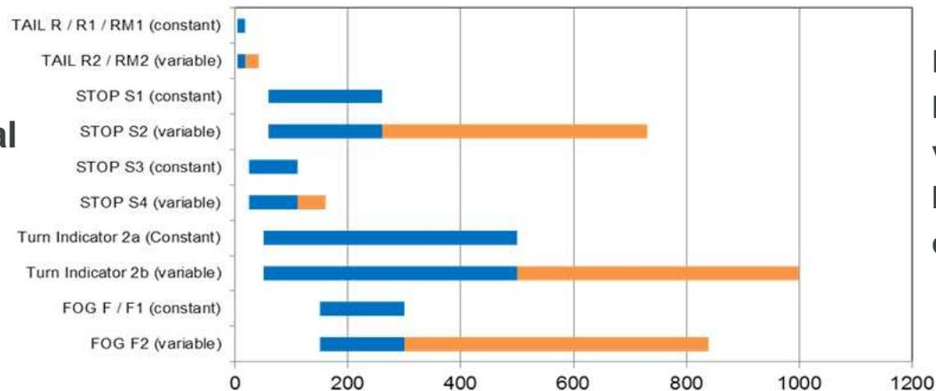
For system with variable light intensity, the maximum value is increased and could be used in poor visibility condition
