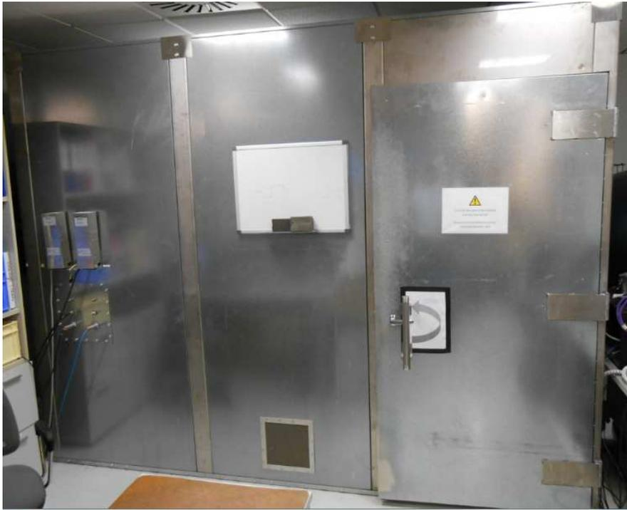
Shielded chamber for EMC testing
