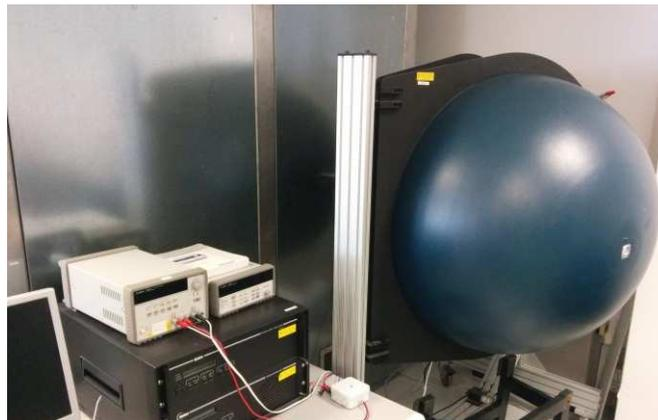
**Integrating spheres for optical simulation**
