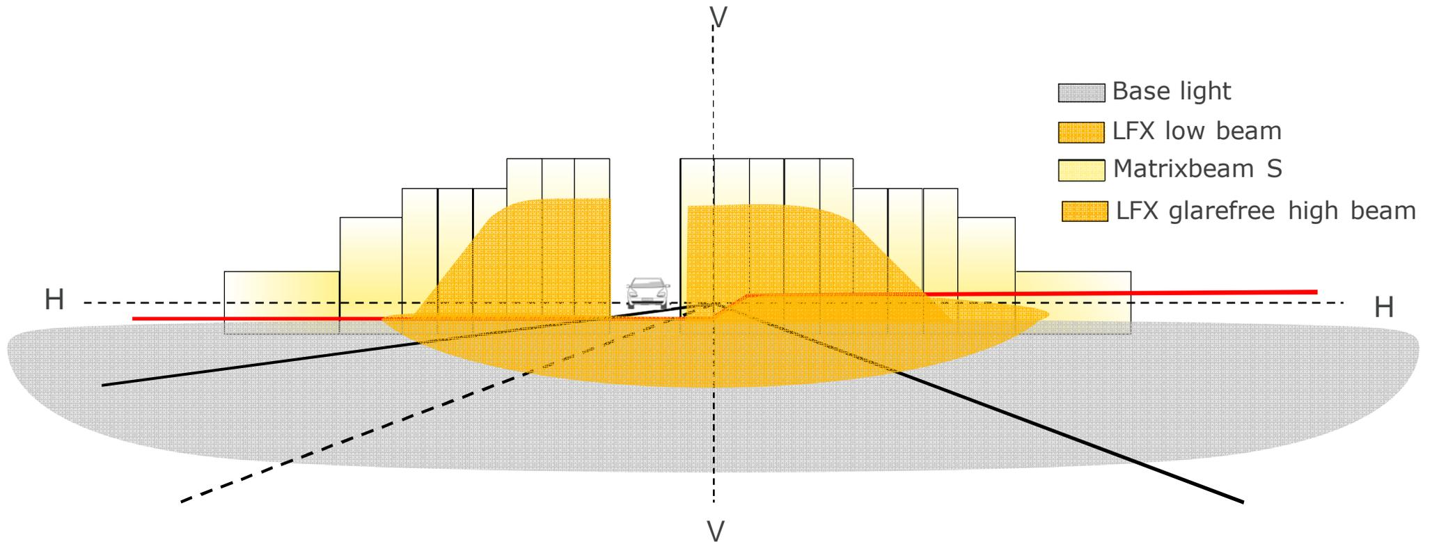
Matrix Beam S : An extension to the conventional partial high beam (LFX in Mercedes S-class)
