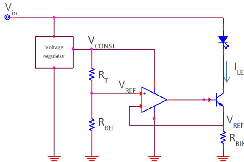
$$V_{REF} = \frac{V_{CONST}}{R_{REF} + R_T} * R_{REF}$$
