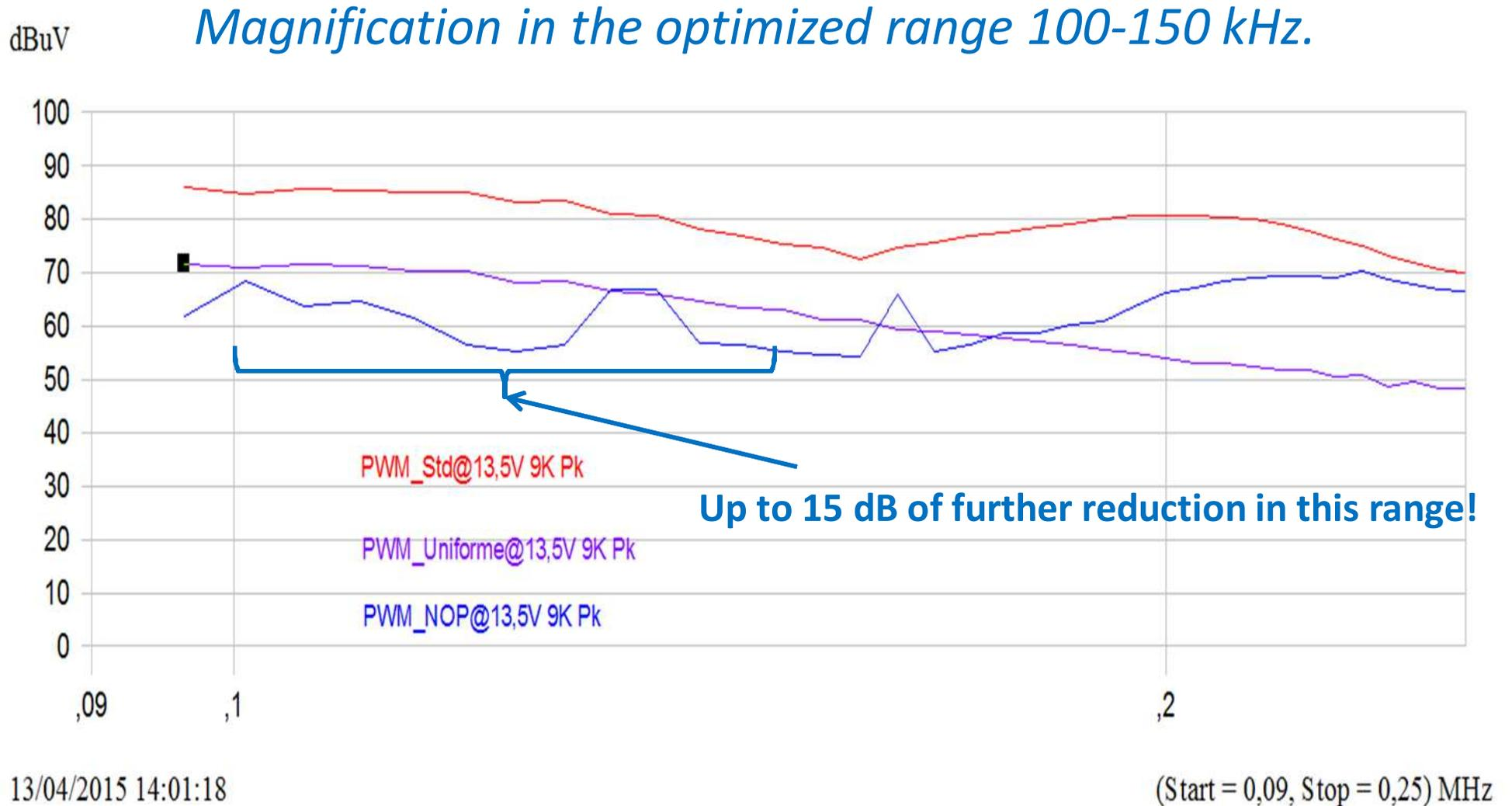
*6 LED branches, 2% PWM without phase shift, with uniform phase shift and with optimized phase shift*
