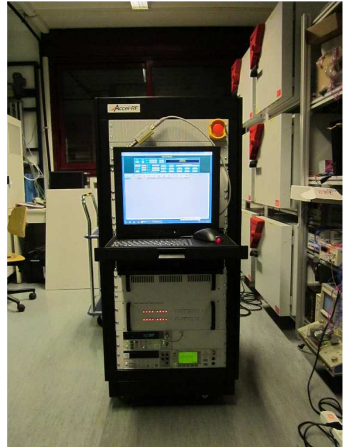
Accel-RF Automated Accelerated Reliability Test Station
