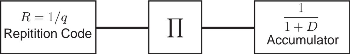
However, if we draw the code graph of a repeat accumulate code, we see that it can just as well be interpreted as a low-density parity check code where the parity checks are degree-2 nodes which can be **recursively** encoded (from right to left).
