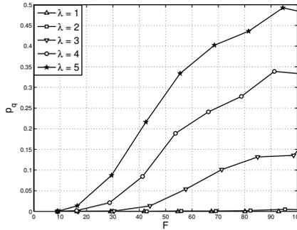
Fig. 3. BN estimation of the probability of buffer overflow  $p_q$  as a function of the number of flows  $\mathcal{F}$  passing through the node.
