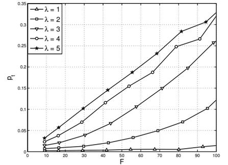
Fig. 4. BN estimation of the probability of transmission failure  $p_t$  as a function of the number of flows  $\mathcal{F}$  passing through the node.
