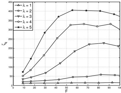
Fig. 2. BN estimation of the average delivery delay  $\zeta_q$  as a function of the number of flows  $\mathcal{F}$  passing through the node.
