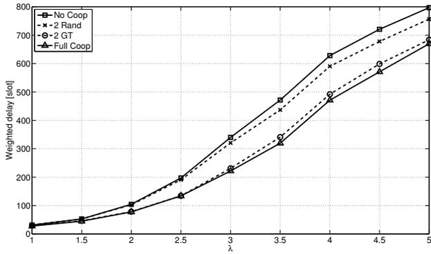
Fig. 5. Weighted delay as a function of the packet generation intensity  $\lambda$ , for the four compared scenarios: with no nodes shared (No Coop); with two nodes shared, randomly chosen (2 Rand); with two nodes shared, chosen via Game Theory (2 GT); and with all the nodes shared (Full Coop).
