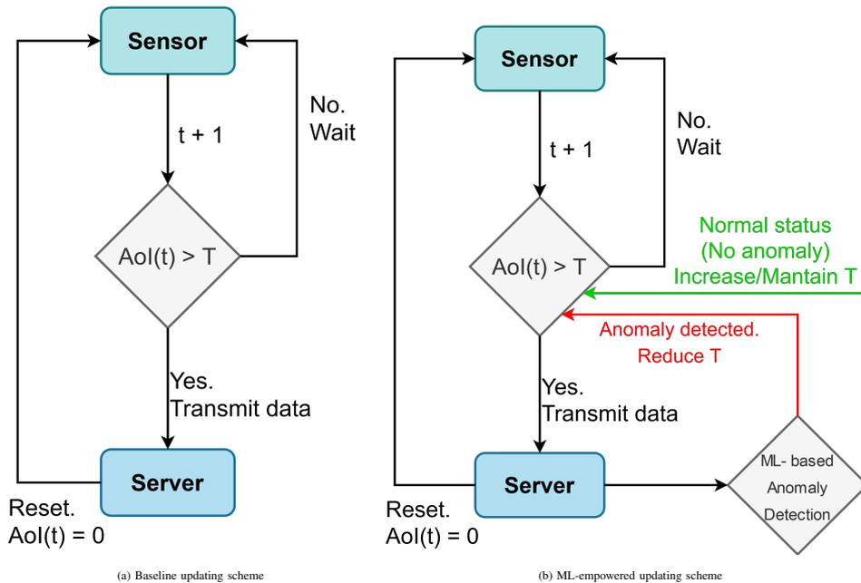
Fig. 1: The role of ML in the AoI evaluations. A baseline scheme without ML (a) is compared with an ecosystem with ML in the loop (b), with a dynamic adjustment of the AoI policies (updating threshold).
