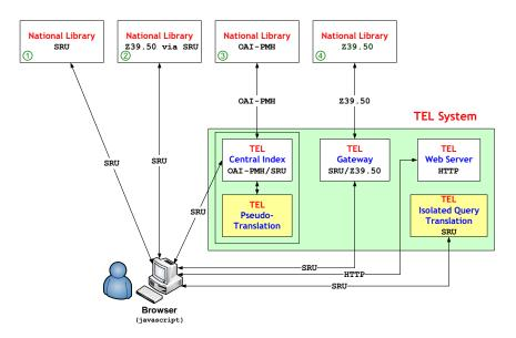
Figure 3: Architecture of the TEL system with new MLIA functionalities.
