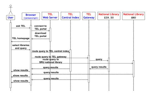
Figure 2: Sequence diagram of the functioning TEL system.
