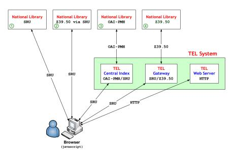
Figure 1: Architecture of the TEL system.
