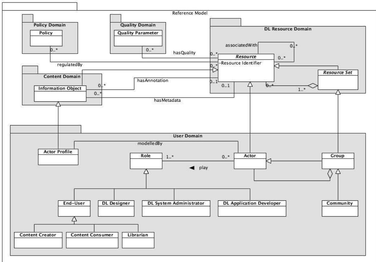
**Figure B-3. User Domain UML Class Diagram**
