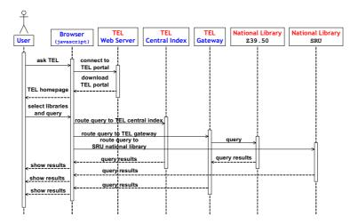
Fig. 2. Sequence diagram of the functioning TEL system
