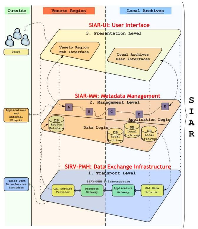
Fig. 1. SIAR Architecture Layers
