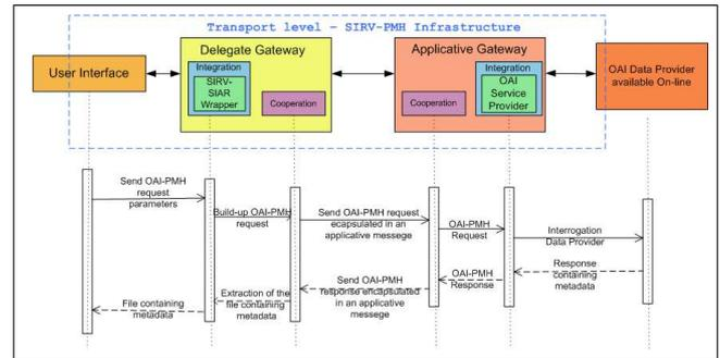
Fig. 2. SIRV-PMH Functioning
