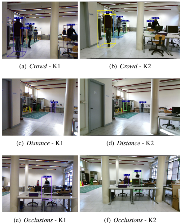
Figure 20: Sample tracking results with Kinect v1 and v2 for the three test videos. For every track, its ID and the distance from the sensor is reported.
