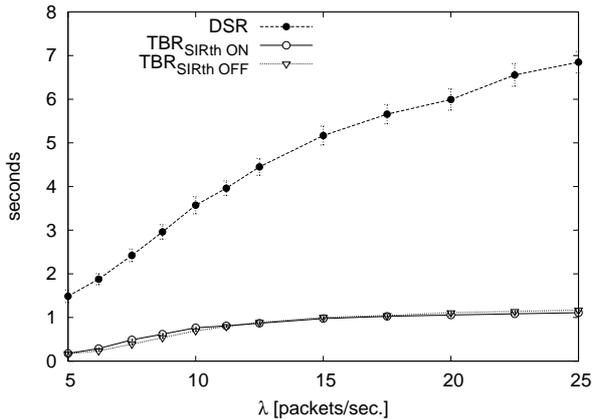
Figure 4: Average end-to-end (nodes → APs) packet delay.
