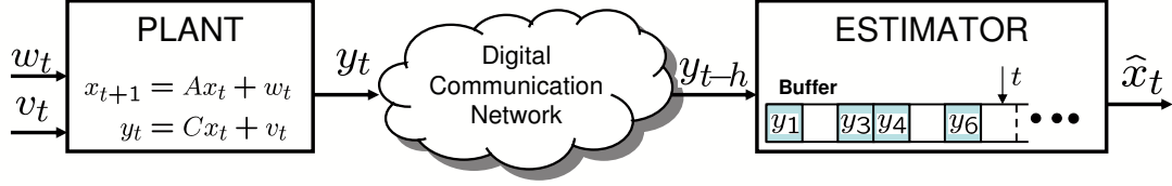
Fig. 1. Networked systems modeling. Sampled observations at the plant site are transmitted to the estimator site via a digital communication network. Due to retransmission and packet loss, observation packets arrive at the estimator site with possibly random delay.
