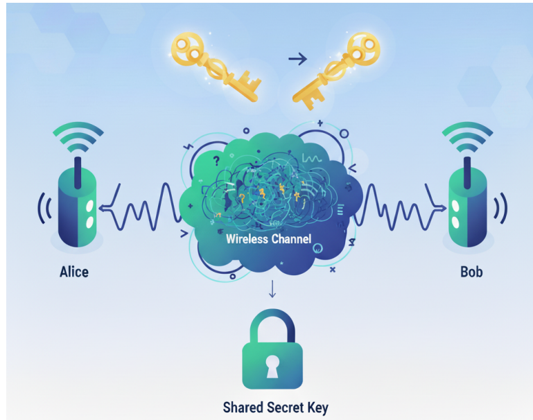
Figure 4.1: An illustration of secret key generation (SKG) system making use of the randomness of the wireless channel.
