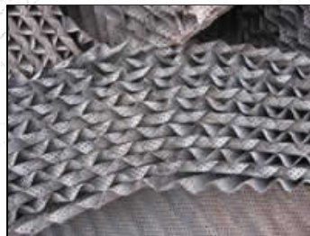
Structured packing (photo courtesy of Paul Phillips)
